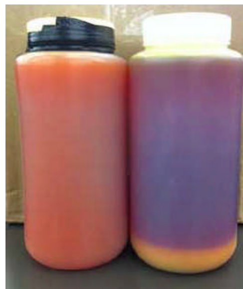
On the left is a non-food grade corn oil immediately after extraction. On the right is the oil after it settles, with only the upper portion being sold as oil. This non-food grade corn oil goes to biodiesel production or feed.
