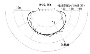
Boundary element method (thin line) and diffuse reflection method (thick line)
